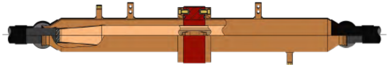
STRAIGHT JOINT (SECTIONALIZED)
